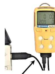
Micro B (5-Pin) to USB cable
