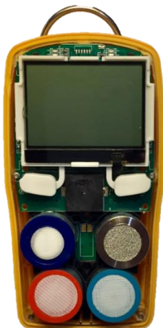
Sensor & LCD replacement
