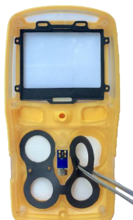
Filter & gasket replacement
