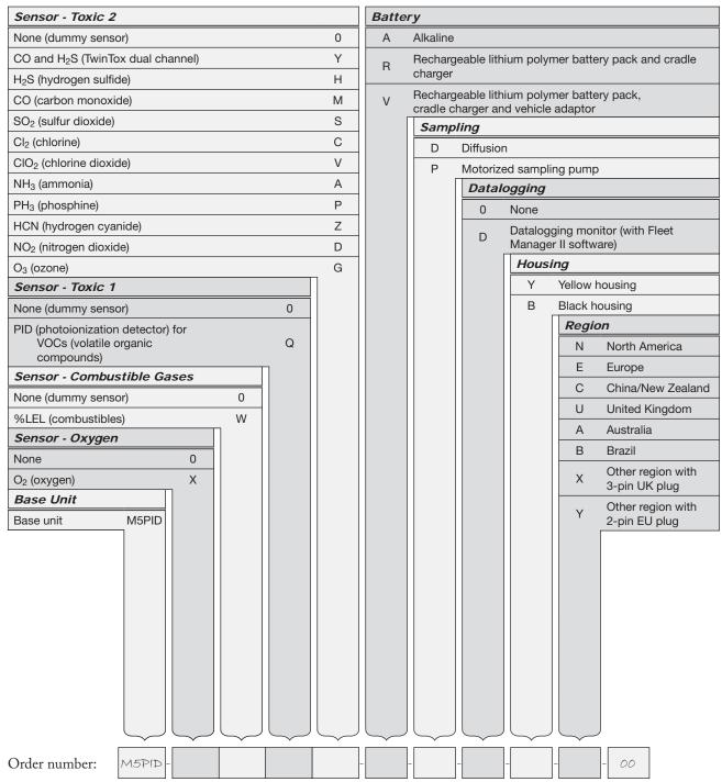
For example, the order number for a GasAlertMicro 5 PID configured for O2, %LEL, VOCs, H2S and CO and equipped with a rechargeable lithium polymer battery pack and cradle charger, motorized sampling pump, datalogging, yellow housing and North American power connectivity would be M5PID-XWQY-R-P-D-Y-N-00.
