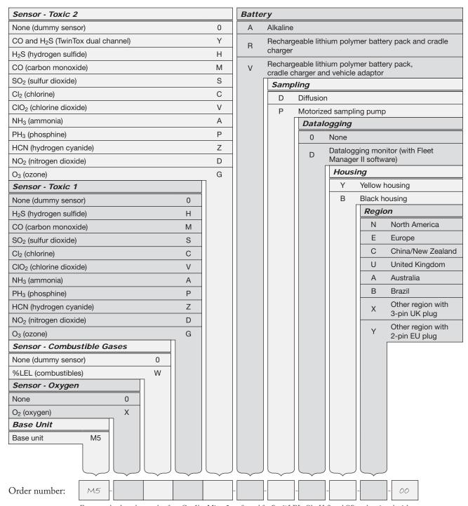
For example, the order number for a GasAlertMicro 5 configured for  $O_2$ , %LEL,  $Cl_2$ ,  $H_2S$  and CO and equipped with a rechargeable lithium polymer battery pack and cradle charger, motorized sampling pump, datalogging, yellow housing and North American power connectivity would be M5-XWCY-R-P-D-Y-N-00.
