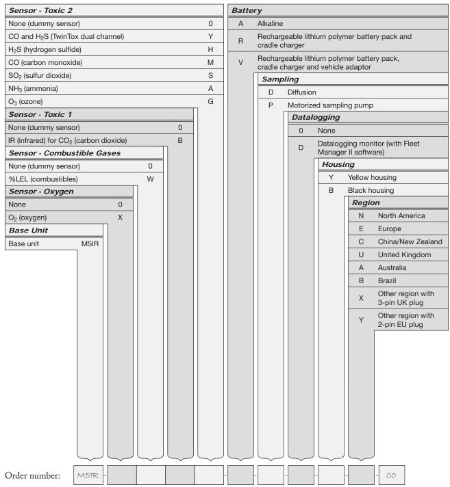
For example, the order number for a GasAlertMicro 5 IR configured for O2, %LEL, CO2, H2S and CO and equipped with a rechargeable lithium polymer battery pack and cradle charger, motorized sampling pump, datalogging, yellow housing and North American power connectivity would be M5IR-XWBY-R-P-D-Y-N-00.
