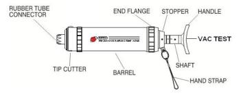
Fig.-1 Uniphos Precision Air Sampling Pump (ASP-40)
