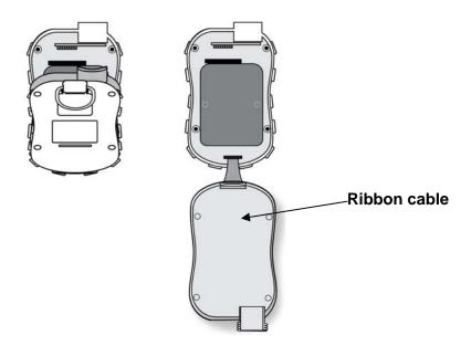
6. Carefully disconnect the battery from the battery connectors on the circuit board by pulling it toward the bottom of the instrument. Be careful not to damage the ribbon cable.
