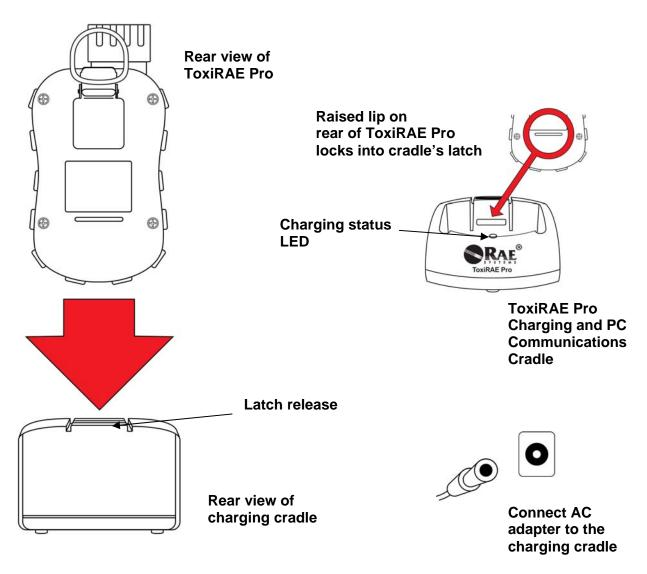
**Note:** Before setting the ToxiRAE Pro into its charging cradle, visually inspect the contacts to make sure they are clean. If they are not, wipe them with a soft, dry cloth. Do not use solvents or cleaners.
