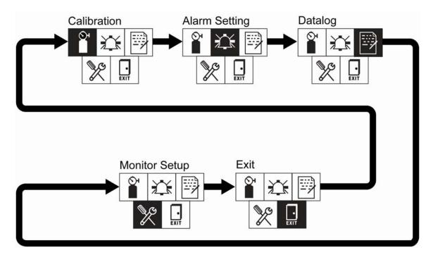
Note: When you reach Exit and press [MODE], the menu cycles back to Calibration.
