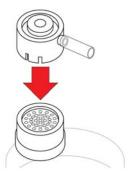
2. Attach the hose from the regulator/calibration gas cylinder to the Calibration Adapter's inlet.
