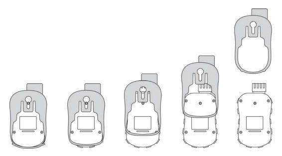
5. Inspect the rubber boot for damage, and replace it if it is cracked or torn.
