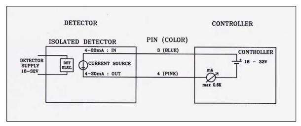
Figure 13: 4-20mA Wiring (Sink Option)
