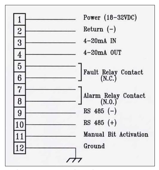
**Figure 10: Connector Interface Option**
