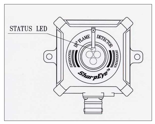
Figure 5: Indication LEDs
