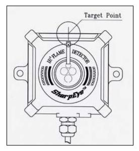
Figure 17: Mini IR3 Detector Target Point
