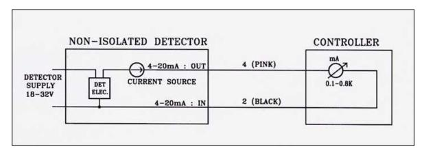
Figure 14: 4-20mA Wiring (Source Option)
