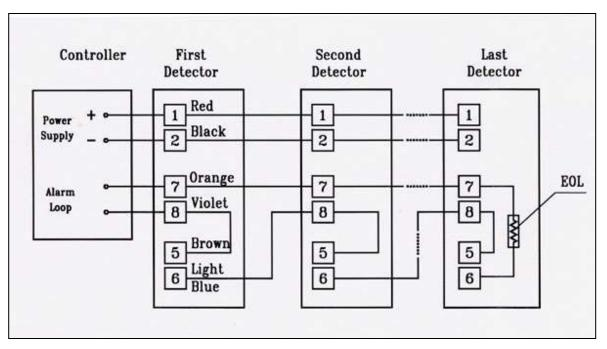
Figure 15: Typical Wiring for 4 Wire Controllers
