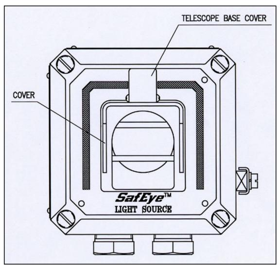
*Figure 1: Light Source – Reflector Type*
