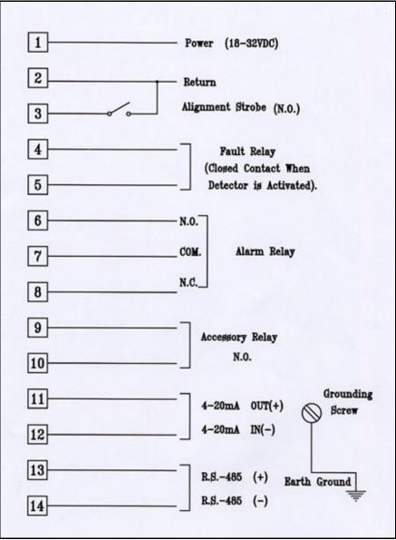
Figure 17. Detector's Wiring Diagram
