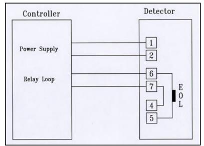
Figure 19. Typical 4 Wire Controller
