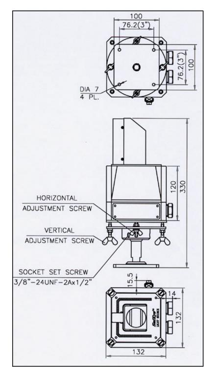
Figure 22. Source Outline Drawing (Reflector Type) With Swivel Mount
