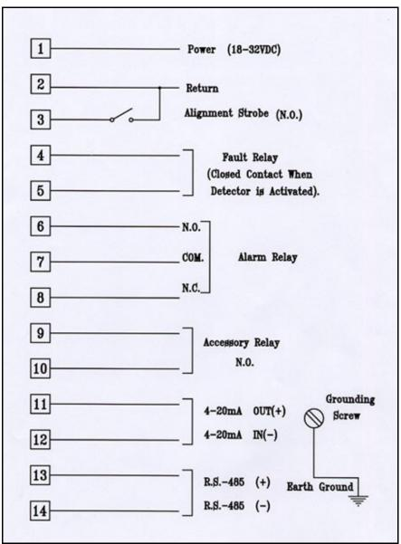
Figure 3. Detector's Wiring Diagram
