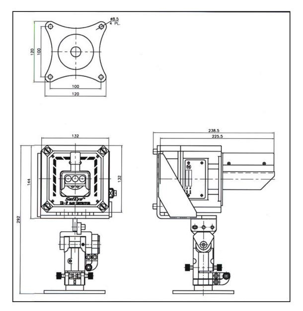
Figure 23. Detector and Tilt Mount Outline Drawing
