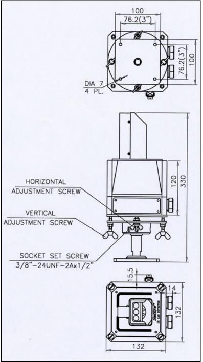
Figure 21. Detector Outline Drawing With Swivel Mount
