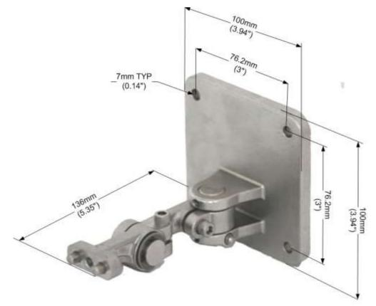
Figure 6 shows the Tilt Mount Assembly with dimension in both millimeters and inches.
