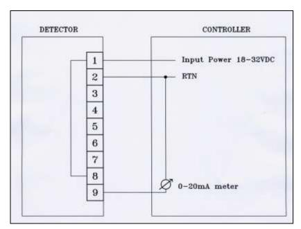
Figure 11: 0-20mA Wiring Option 1 (Converted to Source 3-Wire)
