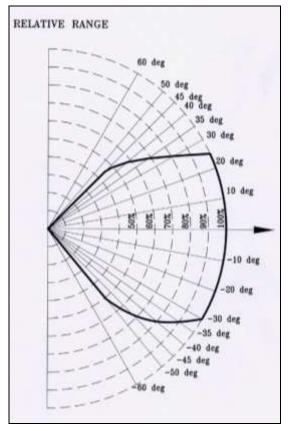
**Figure 2: Vertical Field of View**
