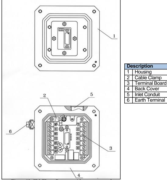
Figure 12: IR3 Flame Detector with cover removed
