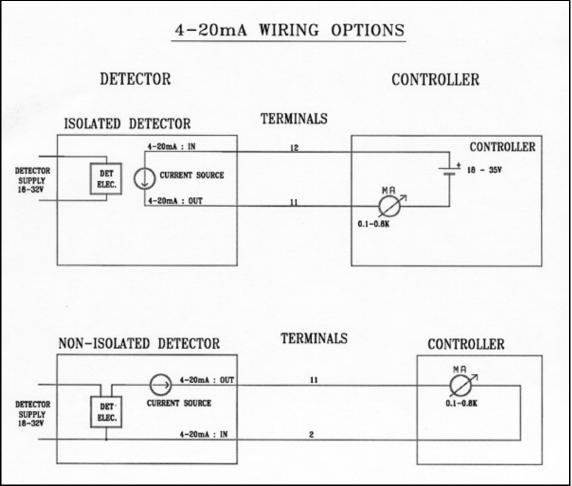
Figure 16: 4-20mA wiring
