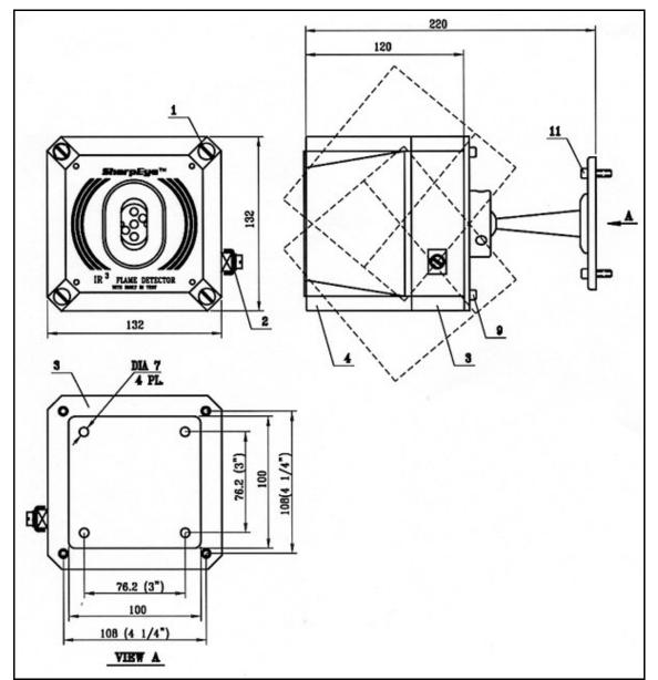
Figure 8: IR3 Detector and Swivel Mount Assembly
