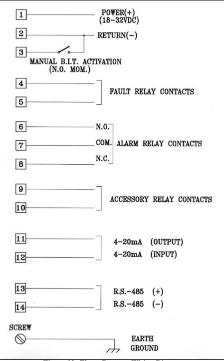
Figure 13: Flame Detector Wiring Diagram
