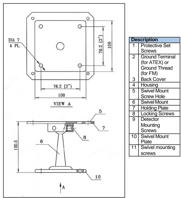
Figure 9: Swivel Mount Assembly - Outline Drawing
