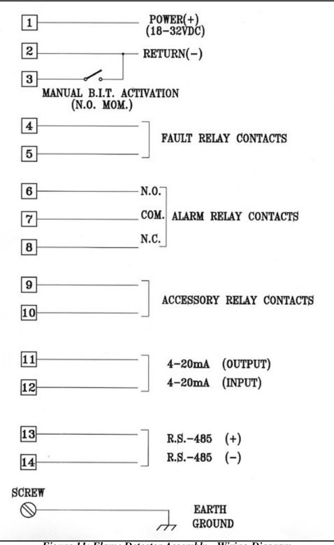
Figure 11: Flame Detector Assembly - Wiring Diagram
