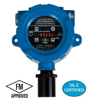
Factory Mutual (FM) Approval for performance, electrical safety and environmental parameters including Class I, Div. 1, Groups B, C, D and Class I, Zone 1, Group IIC, IP66. With a NEMA-4X enclosure standard, approved multiplexing, and approved six month calibration interval, cost of ownership is minimized at the acquisition, installation and operating stages
