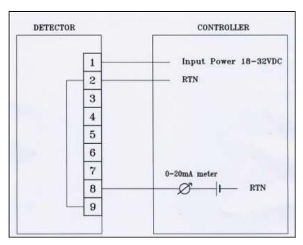
Figure 11: 0-20mA Wiring Option 1 (Unisolated Sink 3-Wire)
