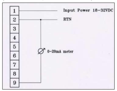
Figure 10: 0-20mA Wiring (Source) 3-Wire Connection
