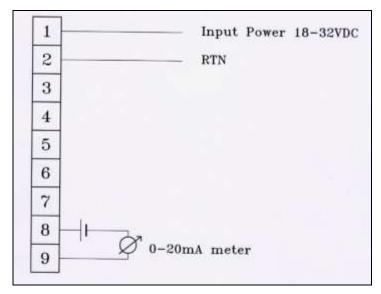
Figure 9: 0-20mA Wiring (Sink) 4-Wire Connection
