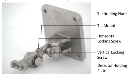
Figure 4: Tilt Mount Assembly
