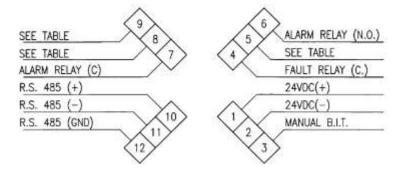
Figure 7: Wiring Terminals
