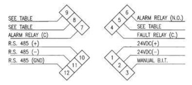
Figure 8: Wiring Terminals
