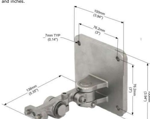
Figure 6 shows the Tilt Mount Assembly with dimension in both millimeters and inches.
