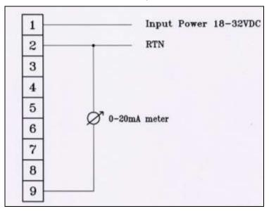
Figure 11: 0-20mA Wiring (Source) 3-Wire Connection
