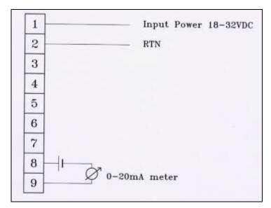
Figure 10: 0-20mA Wiring (Sink) 4-Wire Connection
