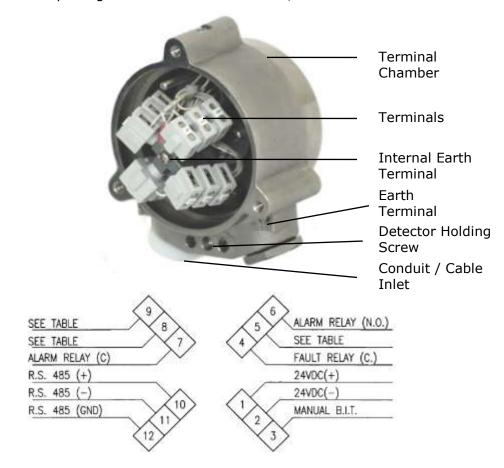
Figure 7: Detector with Cover Removed
