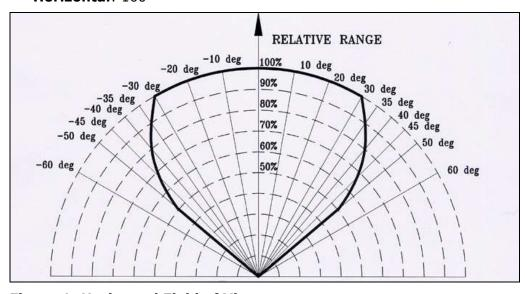
Figure 1: Horizontal Field of View
