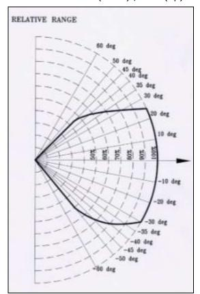
Figure 2: Vertical Field of View
