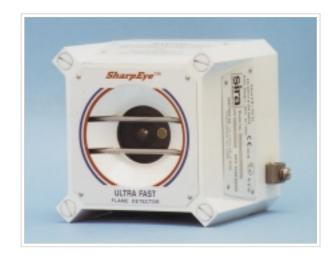
The detector is sensitive to radiation in two frequency ranges of the electromagnetic spectrum: the infra red (IR) and the ultraviolet (UV). Only simultaneous sensing within these two ranges of radiation will result in a detector output pulse.
