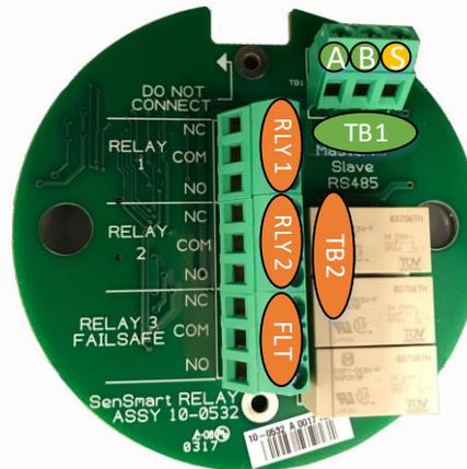
*Figure 5 SensePoint Relay Option Wiring*
