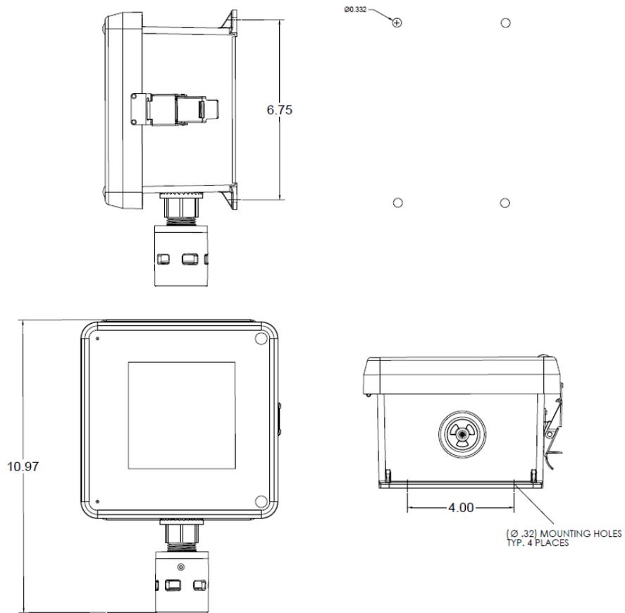
Figure 13 Mounting Dimensions
