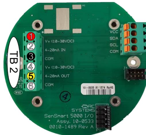
Figure 3 SensePoint Wiring
