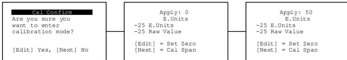
Figure 12 Calibration Menu Flowchart
