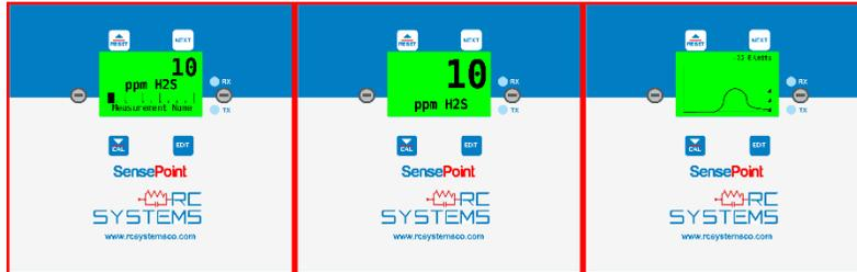
Figure 8 SensePoint Data Display Screens
