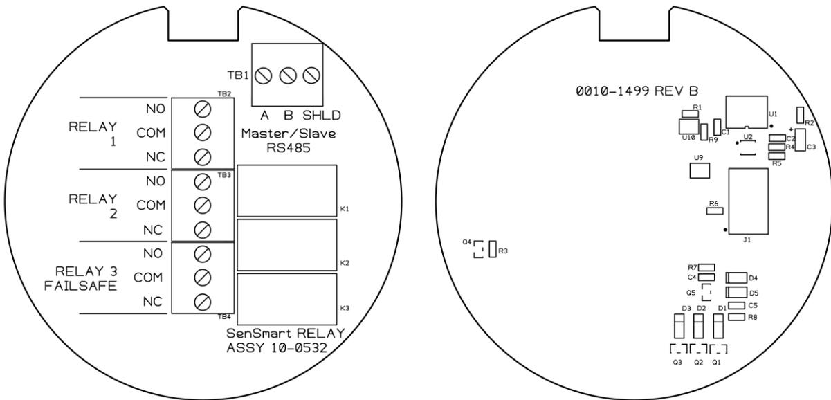
Figure 16 10-0532 Modbus/Relay Board
