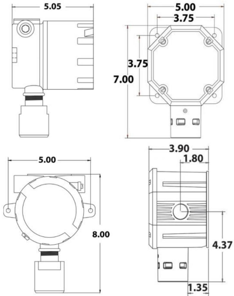
*Figure 2 Remote Sensor Enclosure Mounting Dimensions*
