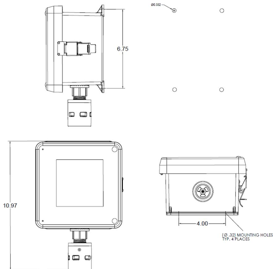
Figure 1 SensePoint Mounting Dimensions
