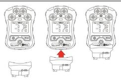
Align the Travel Charger with the middle of the MicroRAE and press it until it is firmly attached.
