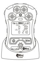
Remove the instrument from the cradle by tilting the release on the rear of the charging cradle away from the instrument and lifting the MicroRAE.
