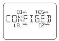
Press [Y/+] to advance through screens that tell you if the radio is on, BLE is on, GPS is on, WiFi is on, etc. These change, depending on the instrument's configuration.
