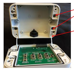
Mount the case to a wall or other flat surface. There are 4ea. through holes for fastening the case.
