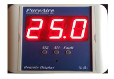
**NOTE:** To fine tune the reading to match the reading on the oxygen monitor, use the "Set 20mA Span" menu. Push the joystick up or down until both displays match.
