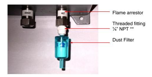
The *Air Check*  $\checkmark$  *Ex* monitor is a sample draw type. The internal sample pump flow rate is programmed at the factory and cannot be changed in the field. A flow sensor on the relay board continually monitors flow rate. When a loss of flow is detected, a signal is sent to the fault relay and the front mounted LED will activate. Sample flow to the monitor is continuously monitored and controlled by the flow control microprocessor.
