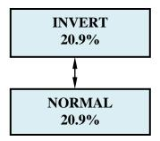
After entering the relay state the display will default back to the Set Relay 2 Alarm Threshold menu. The display will scroll the following:
