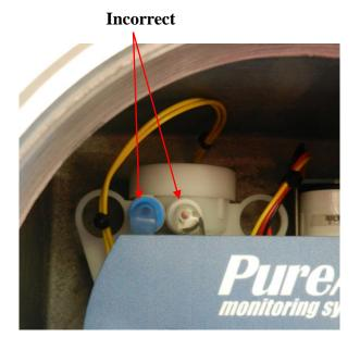
Please make all wiring terminations to the monitor and reassemble the electronics inside the enclosure before powering the monitor. Shorting any wiring to the metal enclosure will blow the internal fuse and void your warranty.
