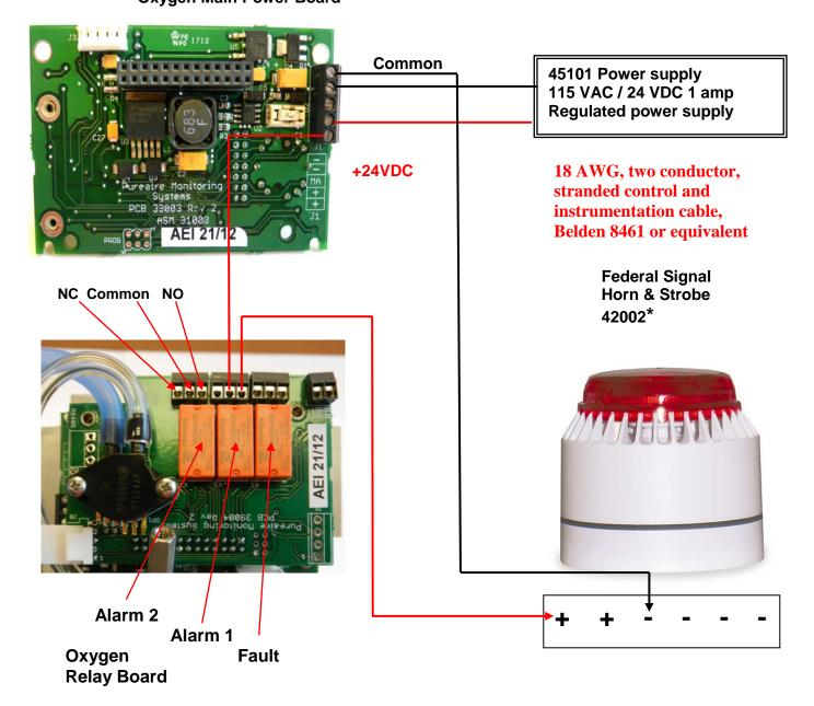
This drawing shows how to connect a remote Horn and strobe to PureAire's Oxygen monitor with the Alarm relay #1 set to a Normally Open position.
