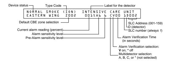
Figure 4.1 Sample Detector Read Status Display
