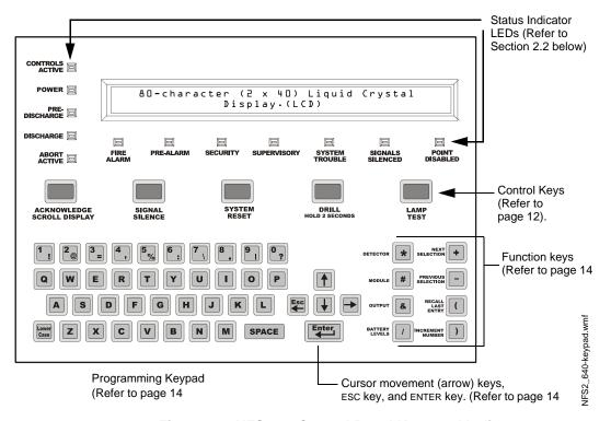
Figure 2.1 NFS-320 Control Panel Keys and Indicators
