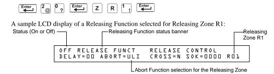
Figure A.1 Sample Read Status for a Releasing Zone
