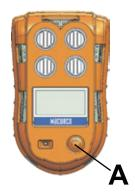
As a safety feature, if gas is detected while in a menu, the MG-1 will revert back to the home screen to ensure the gas readings are displayed. This will not occur if the MG-1 was in bump test mode, calibration mode or peak mode.
