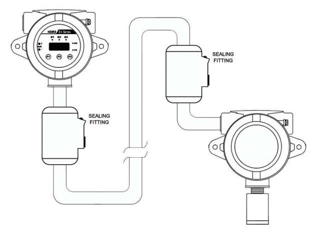
The Smart Sensor Head can be equipped with EX Series locally or remotely. For installations where the smart sensor head assembly will be mounted remotely from EX Series, the max distance between EX Series and Remote Smart Sensor Head is 100 meters. The Remote Smart Sensor Head Assembly is not included in the EX Series standard package, it must be ordered separately.
