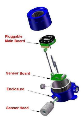
Important: Calibrate the transmitter whenever a component is replaced. But if you replace a smart sensor assembly with a sensor onboard from Macurco, you don't need to recalibrate the transmitter, as all the calibration information has been stored in the smart sensor board in factory process.
