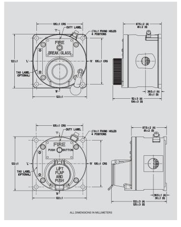
Both the Exia units and the Exd units have the same external appearance. Also the internal components are identical throughout the range. Each unit can be wired for either NO, NC or CO contacts to customer specification.
