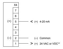
4-20 mA, 2-wire loop-powered sensor/transmitter
