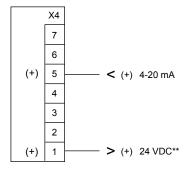
Twisted, shielded wire is recommended for 2- or 3- wire configurations.
