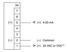
4-20 mA, 2-wire loop-powered sensor/transmitter
