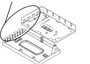
Once lid is closed, back out set-screw to secure enclosure cover
