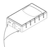
Once lid is closed, insert set-screws to lock enclosure. Requires 1/16" Allen wrench
