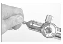
Connect either end of the calibration tubing to the regulator's nipple.
