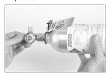
Holding the regulator, turn the calibration gas cylinder in a clockwise direction to tighten.
