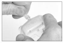
Connect the other end of the tubing to the calibration cup.
