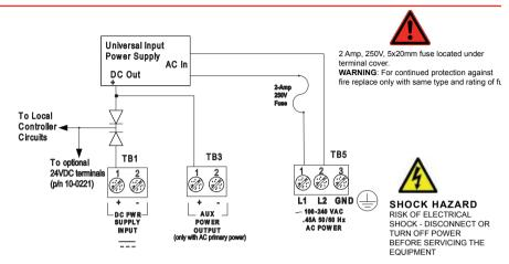
Figure 3-1. DC Power Supply Schematic
