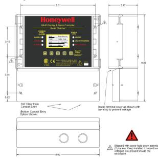
Figure 4-1. NEMA 4X Wall Mount Enclosure
