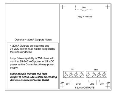
Figure 3-6. Optional Optional 4-20mA Analog Output Board (P/N 10-0308)
