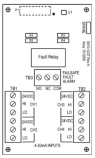
Figure 3-3. Optional Analog Input PCB (P/N 10-0221)
