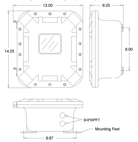
Figure 4-2. NEMA 7 Explosion-Proof Wall Mount Enclosure
