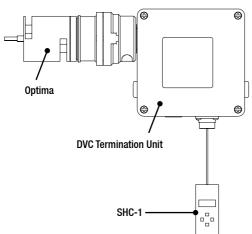
When used for calibration and diagnostics purposes the Hand-Held Interrogator SHC-1 allows digital communication with the Optima. It is connected to the Optima via the IS Socket on the Termination Unit DVC100 or via the SHC Protection Device for other junction boxes.
