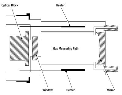
Searchpoint Optima Plus uses the dual wavelength infrared absorption principle to detect hydrocarbon gases and vapours in various concentration ranges. The instrument measures the number of molecules of the target gas in the light path, which depends on the concentration of the target gas. In addition to the relatively long and open measuring chamber, Searchpoint Optima Plus can be fitted with a short enclosed flow through-cell as part of the chassis.
