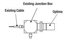
Replacing existing Sensor using existing Junction Box and Cable (where suitable).
