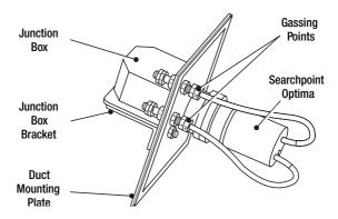
Notes: 1. In order to make use of the gassing points provided, the Optima unit must be fitted with the Remote Gassing Cell (2108B0240).
