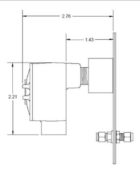
The duct mounting kit is assembled and installed onto a duct as below:-
