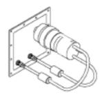
(6) Secure the mounting plate to the duct.
