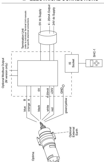
Configuration for Termination Unit with IS Socket and Hand-Held Interrogator
