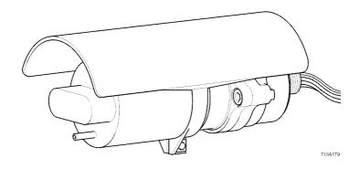
**Gassing Cover Fitted Over Weather Protection**
