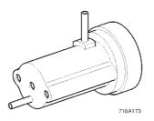
Used to achieve accurate calibration of Optima Plus on the bench. Requires all protective covers and attachments to be removed from the measurement chamber except for the dust barrier. The calibration procedures are described in Section 6.
