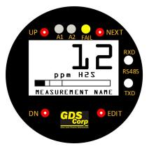
Activating DOWN/CAL, followed by EDIT, while in display mode initiates calibration mode. For the balance of this manual, the term "press" will be used to describe activation of any key via the magnetic wand.
