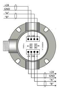
Figure 5-7: MODBUS Wiring Junction Box
