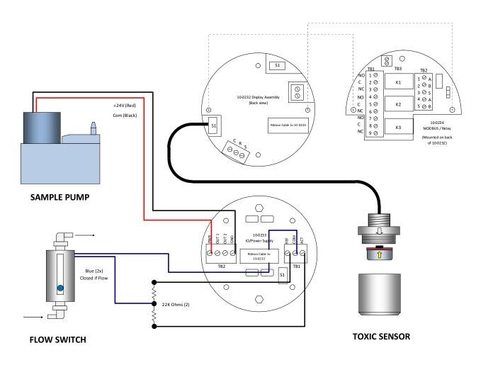
Figure 14-1: GDS-58XP Wiring Diagram (Toxic Sensor)
