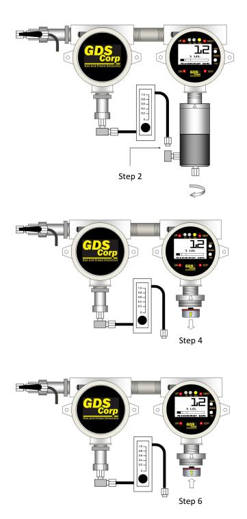
Step 1: If necessary, declassify area or remove power Step 2: Disconnect the sample inlet tube to the sensor flow cell Step 3: Unscrew the sensor flow cell and sensor head cover
