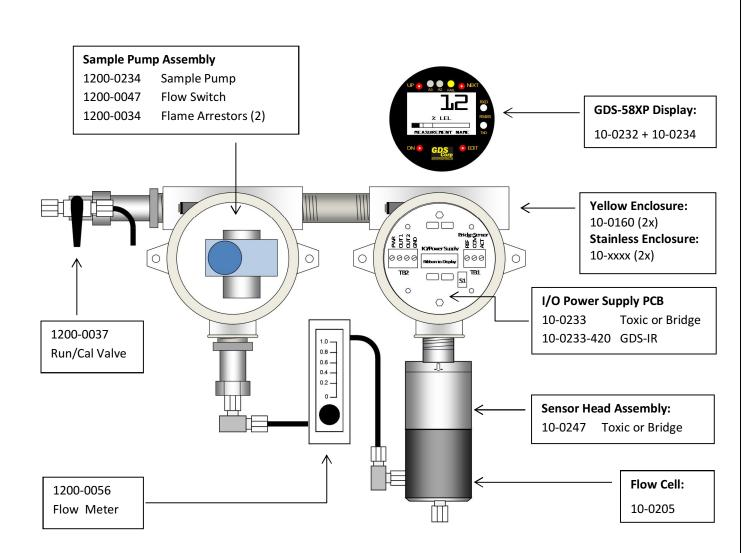
Figure 12-1: GDS-58XP Assembly with Toxic / Bridge Sensor (Spare Parts)
