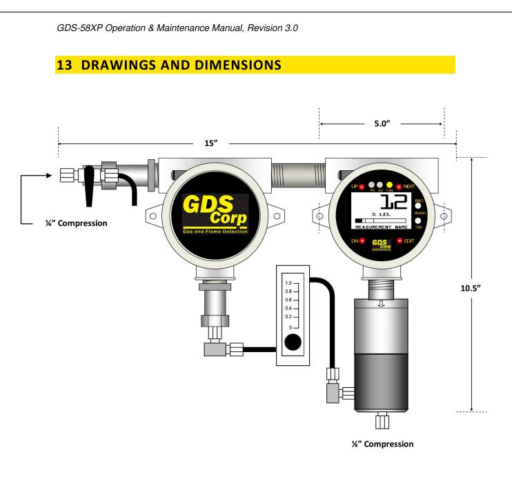
Figure 13-1: GDS-58XP Dimensions (Aluminum Enclosure)
