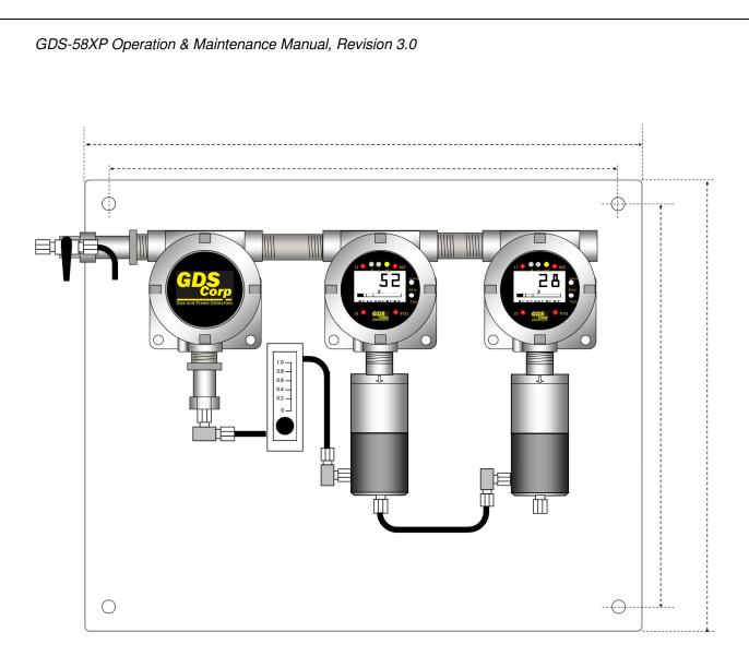
Figure 13-5: GDS-58XP 21" x 17" Mounting Plate Dimensions (SS Enclosures)
