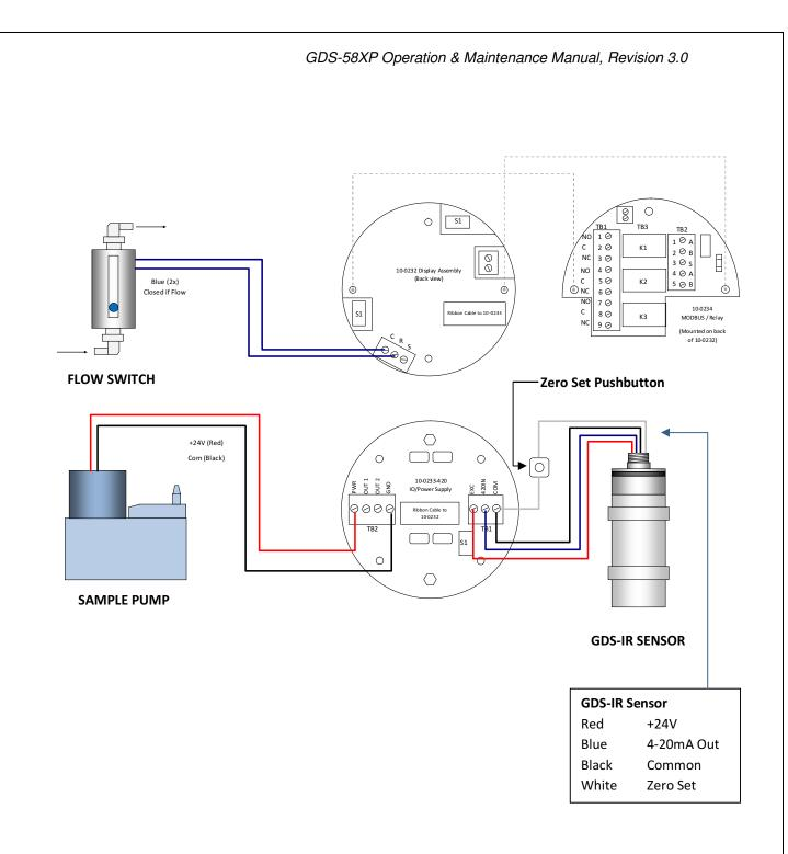
Figure 14-3: GDS-58XP Wiring Diagram (GDS-IR Sensor)
