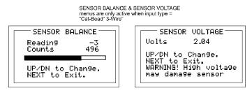
Figure 9-3: Sensor Balance & Voltage Set Menu
