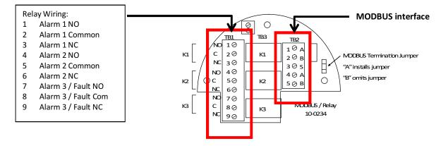
Figure 5-5: RELAY / MODBUS Connections
