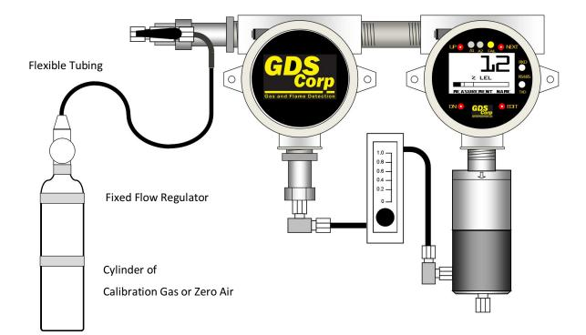
Figure 6-1: GDS-58XP Calibration Setup
