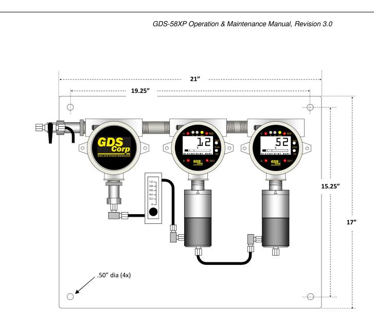
Figure 13-4: GDS-68XP 21" x 17" Mounting Plate Dimensions (AL Enclosures)
