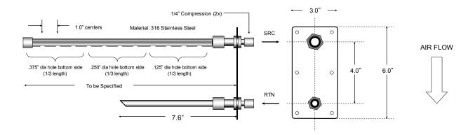
Figure 15-1: Sample Draw Duct Assembly
