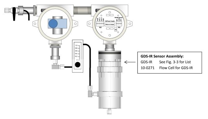
Figure 12-3: GDS-58NXP Assembly with GDS-IR (Spare Parts)
