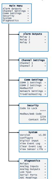
**Alarm Output Menu** – contains settings that control the four optional alarm relays (if installed). These setting include relay programming, on and off delay, failsafe mode and specific input override.
