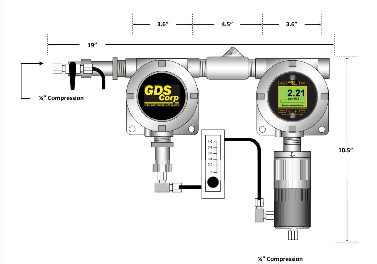
Figure 13-2: GDS-58NXP Dimensions (Stainless Steel Enclosure)
