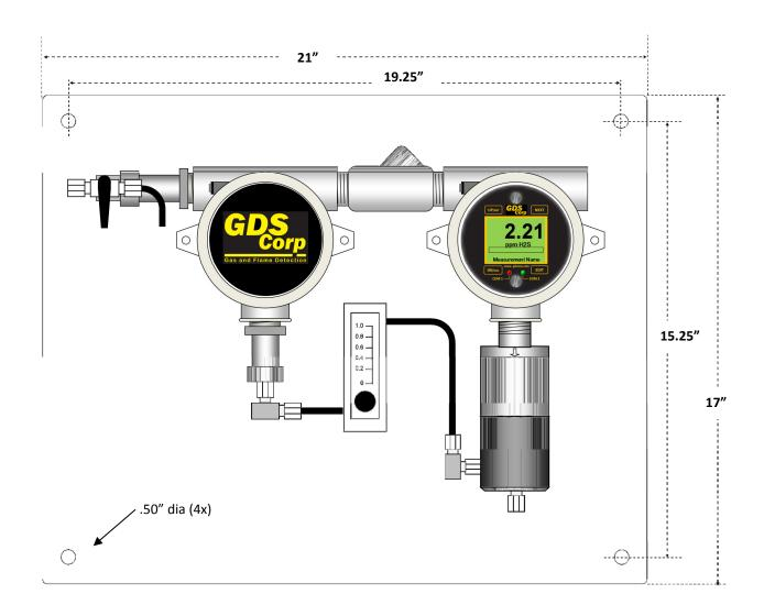
Figure 13-4: GDS-58NXP 21" x 17" Mounting Plate Dimensions
