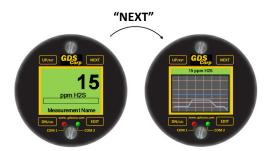
Figure 5-2: Single Channel Display Sequence
