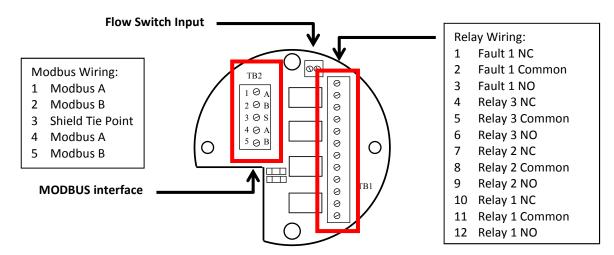
Figure 4-2: RELAY / MODBUS Connections
