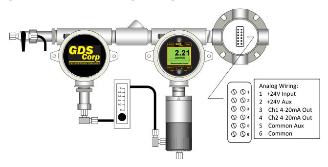
Figure 4-3: GDS-58NXP with Optional Analog Wiring Junction Box (RWJB)
