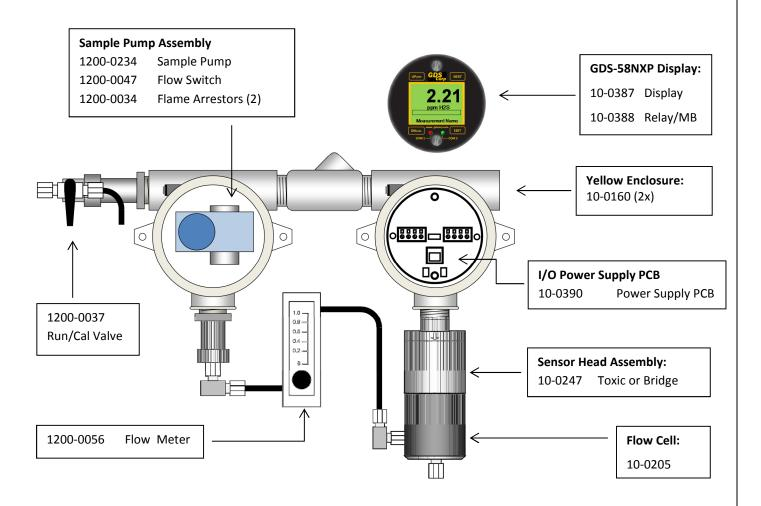
Figure 12-1: GDS-58NXP Assembly with Toxic / Bridge Sensor (Spare Parts)
