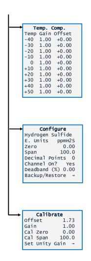
Temperature Compensation compensates for changes in sensor output (gain) and zero value (offset) as sensor temperature changes. Individual values for gain and offset can be entered for eleven points ranging from minus 40C to +60C. Gain and offset values are linearly interpolated between points by the internal microprocessor.
