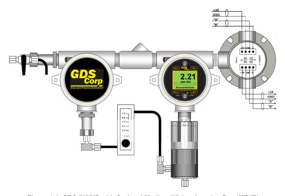
Figure 4-4: GDS-58NXP with Optional Modbus Wiring Junction Box (MBJB)
