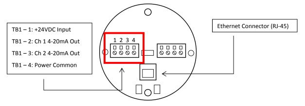
Figure 4-1: GASMAX CX I/O Board
