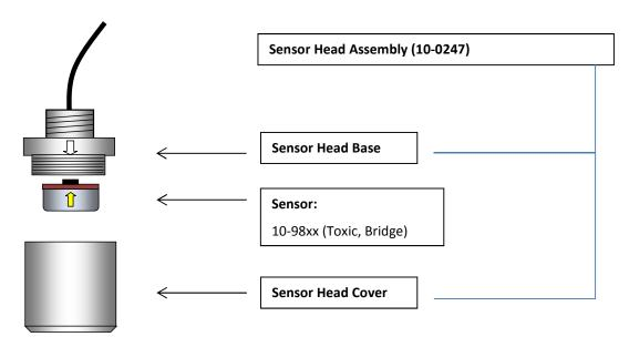
Figure 12-2: GDS-58NXP Standard Sensor Head Exploded View
