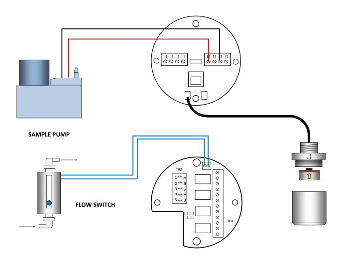
Figure 14-1: GDS-58NXP Wiring Diagram
