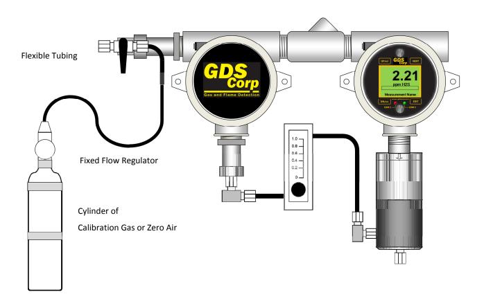
Figure 6-1: GDS-58NXP Calibration Setup
