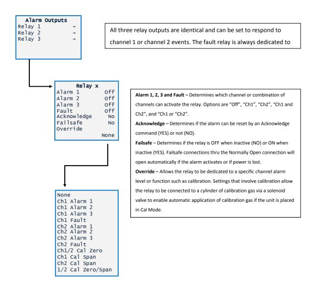
Figure 10-2: Alarm Outputs Menu Tree
