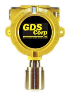
sensor transmitter designed specifically to detect combustible hydrocarbons or carbon dioxide gas. The GDS-50 sensor transmitter 4-20mA output is compatible with the C1 *Protector*, C2 *Protector*, C2 *Quad Protector or C64 Protector* Controllers, the GASMAX II or GASMAX CX gas monitors or any other device with a 4-20mA input and built-in calibration capability.
