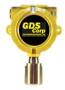
The GDS-48 is a three-wire remote sensor for combustible, carbon dioxide or volatile organic compounds that provides a low impedance bridge-style output suitable for long distance transmission to an appropriate receiver device such as a C1 *Protector*, C2 *Protector*, C2 *Quad Protector* Controller or GASMAX II gas monitor.
