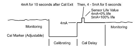
Figure 7-3: SENSOR LIFE TRANSMISSSION FORMAT
