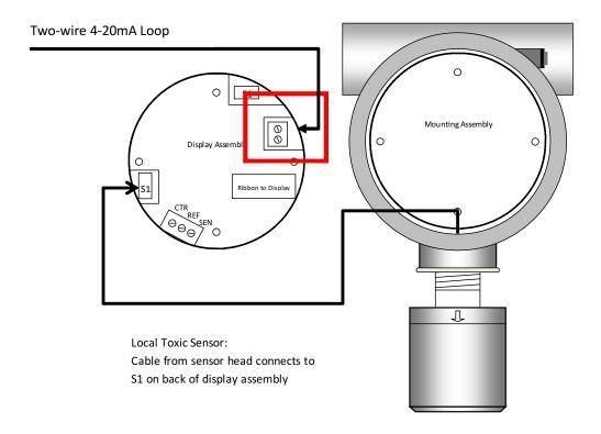
Figure 4-3: GASMAX EC Loop Power Wiring
