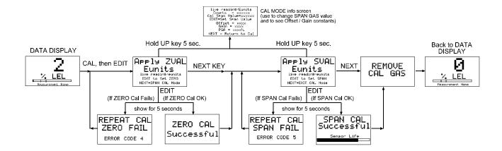
Figure 5-2: CALIBRATION FLOWCHART
