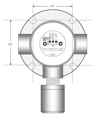
Figure 4-2: GASMAX EC Remote Sensor
