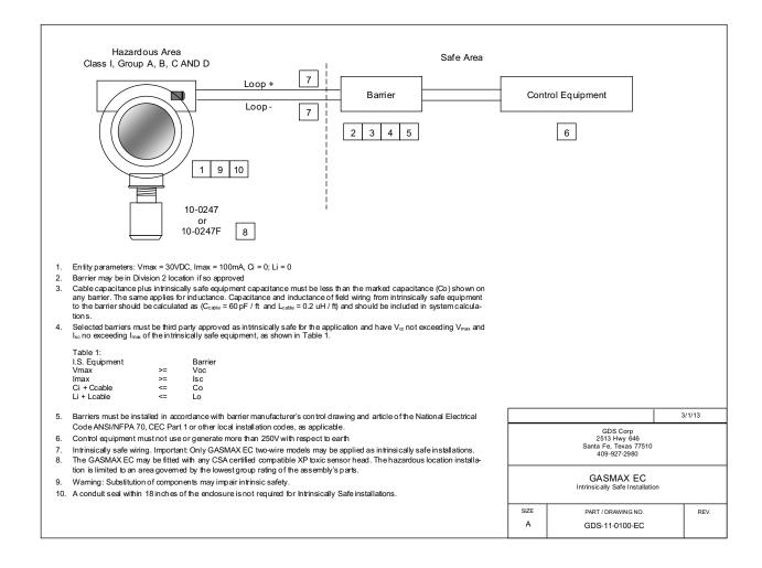
Figure 4-6: GASMAX Intrinsically Safe Installation
