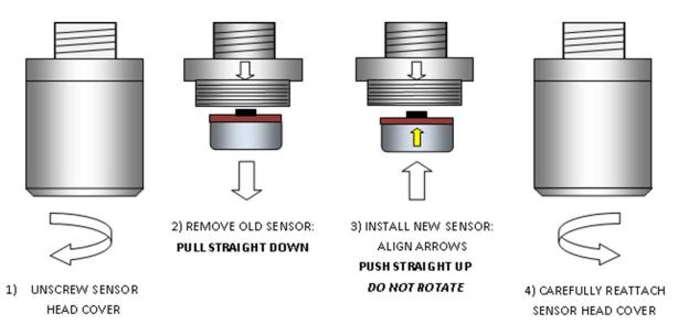
Figure 6-4: Sensor Replacement
