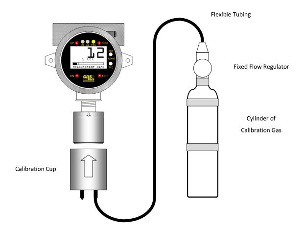
Figure 5-1: Calibration Setup
