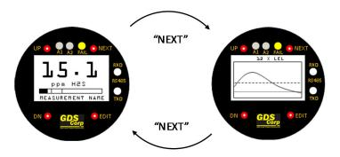
Figure 6-1: GASMAX EC Display Screens
