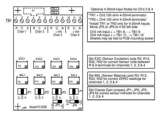
Figure 6-5: 10-0309 Bridge Input Board
