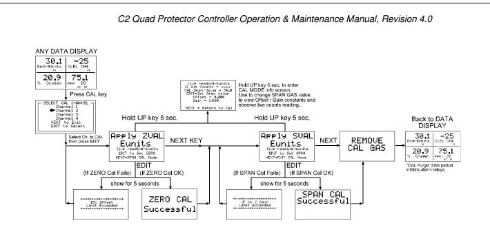
Figure 9-1: C2 Quad Protector Calibration Flowchart
