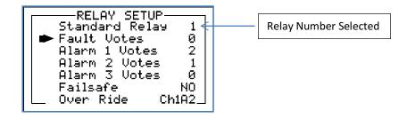
Figure 11-8: Relay Setup Menu
