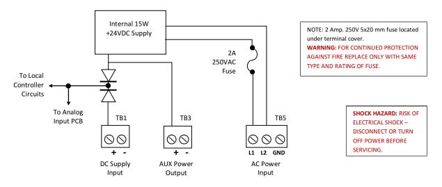
Figure 5-1: Power Supply Input Detail
