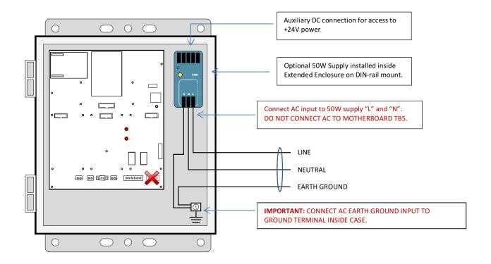
Figure 6-10: Optional 50W Power Supply Wiring
