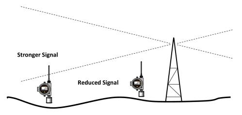
Figure 10-2: Effect of GASMAX Proximity to C2 Quad Protector
