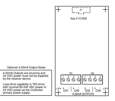
Figure 6-6: 10-0308 Analog Output Board
