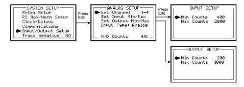
Figure 11-11: Analog Setup Menu
