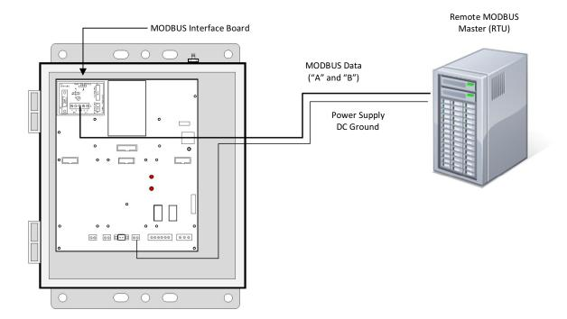
Figure 7-7: Wired MODBUS Slave Output
