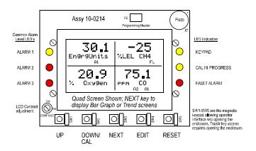
Figure 6-3: Display / CPU Module
