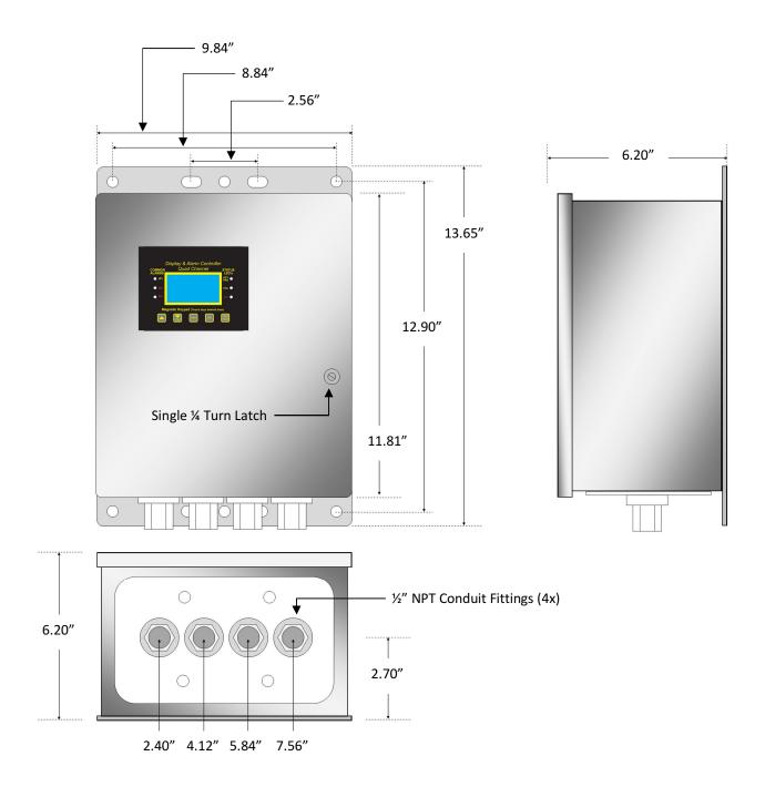
Figure 15-4: NEMA 4X Stainless Steel Enclosure
