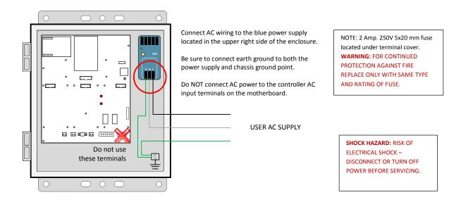
Figure 5-3: Power Supply Input Detail
