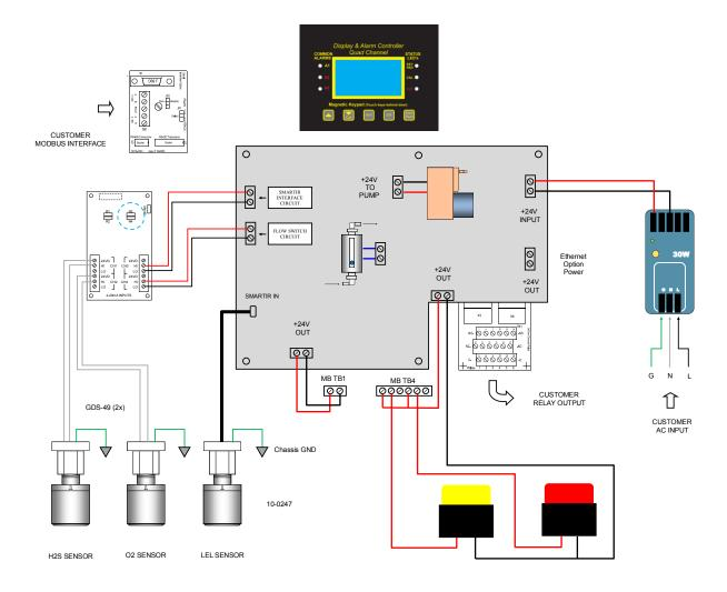
Figure 4-3: C2-WWT Triple-Gas Sample Draw Wiring Diagram
