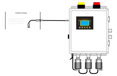
Figure 5-2: Sample Draw with Ambient Exhaust
