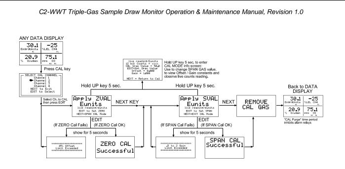
Figure 7-7-1: C2-WWT Calibration Flowchart
