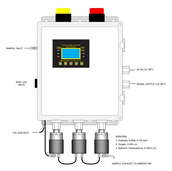
Figure 4-1: C2-WWT Triple-Gas Sample Draw Monitor
