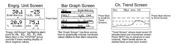
Figure 6-2: C2-WWT Data Display Screens
