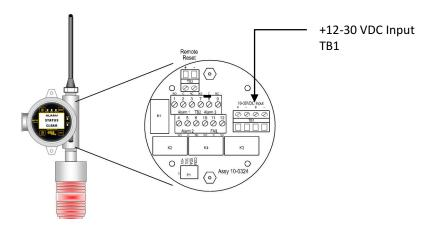
Figure 4-1: DC Power Input Wiring
