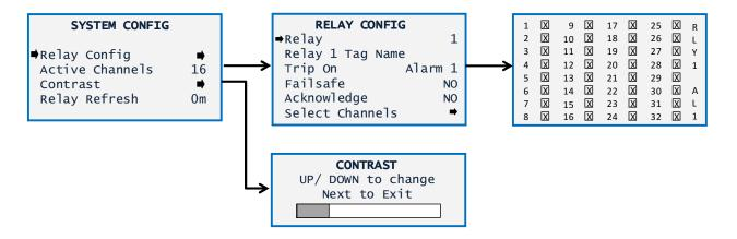
Figure 7-3: System Configuration Menu
