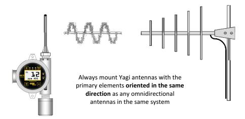
Figure 4-4: Yagi Directional Antenna
