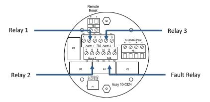
Figure 4-3: 95/TX Alarm Relay Connections
