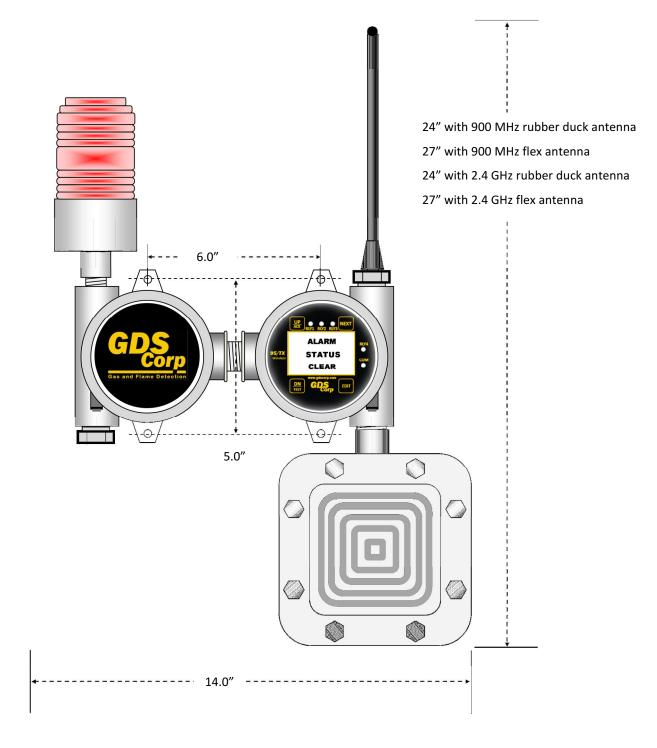
Figure 10-3: 95/TX Dimensions (XP Horn + Strobe)
