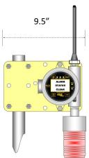
In all cases, the 95/TX enclosure must be properly connected to earth ground to maximize radio reception and as protection against electrical discharge and lightning strikes.
