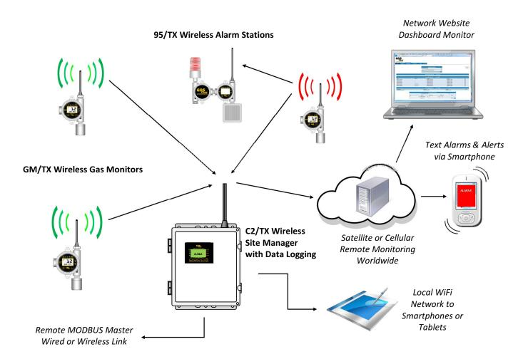
Figure 2-1: GDS Corp Wireless Gas Detection System
