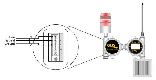
Figure 4-2: AC Power Input Wiring
