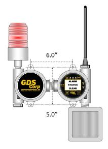
The dual-enclosure unit can also be mounted using the p/n 20-0165 pole-mounting kit as shown at right. For best protection against lightning or electrical discharge, make sure the pole is buried at least 3' into the ground or is properly bonded to earth ground using large diameter wire or braided cable. If the pole extends above the level of the antenna as shown, the pole will provide some additional protection against direct lightning strikes.
