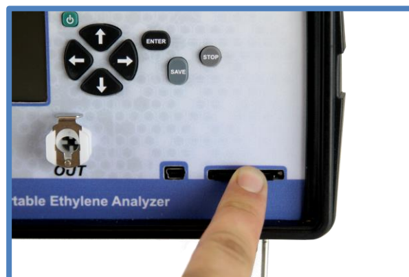
Figure 2: The removable SD card on the F-900 makes data transfer quick and simple.
