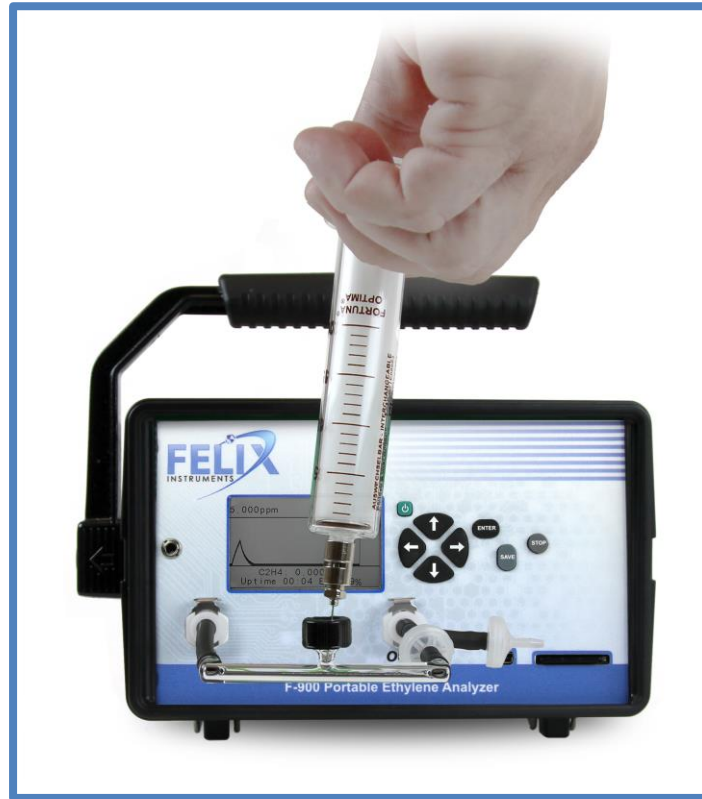
Figure 13: GC emulation port connected to front of instrument for small volume samples.
