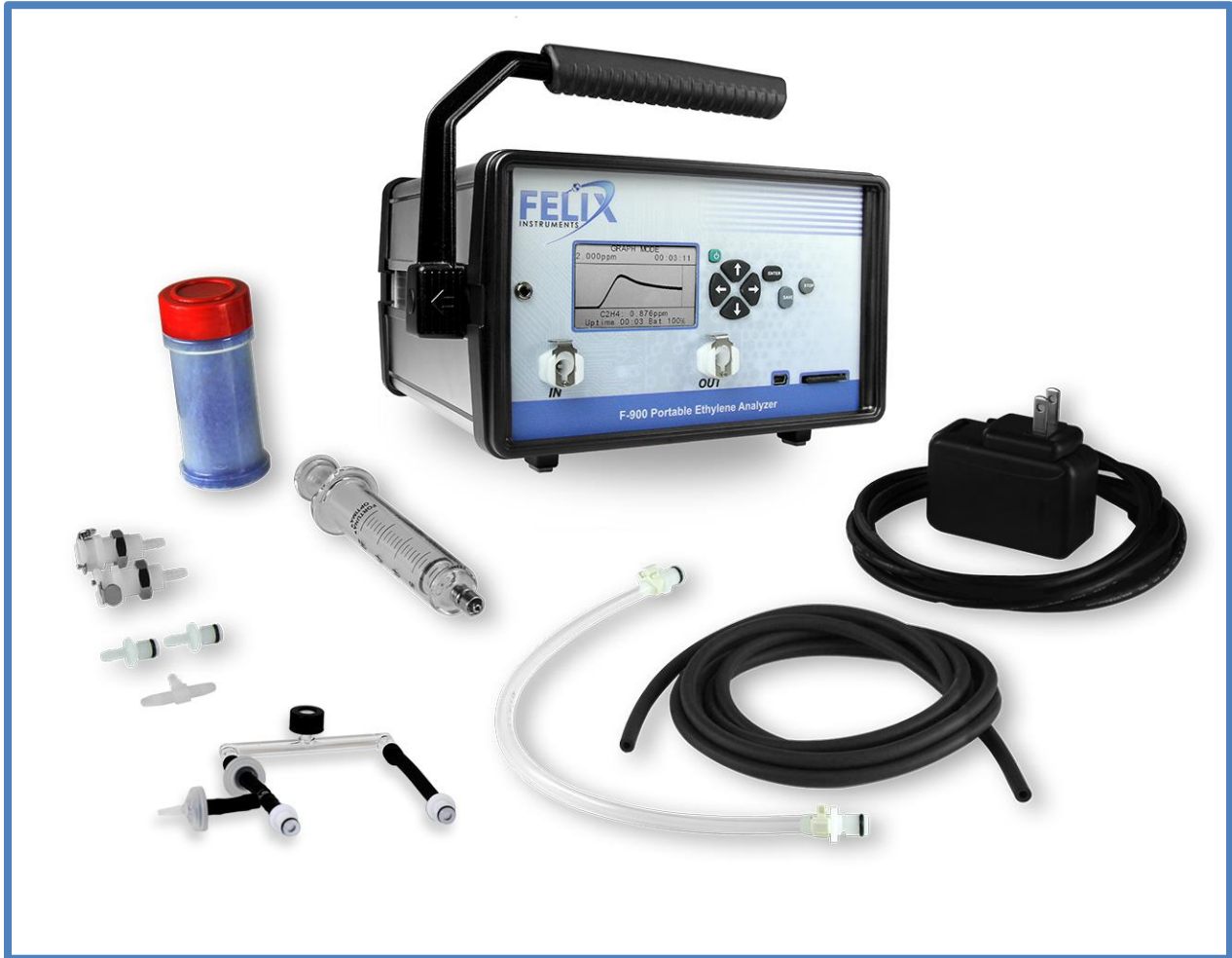
Figure 6: Accessories and parts that arrive with the F-900, clockwise from top center: F-900 ethylene analyzer, power supply and heavy duty USB cable, Viton tubing, Teflon tubing with quick connects, GC emulation port, assorted quick connects, GC emulation sampling syringe, Silica gel in conditioning chamber
