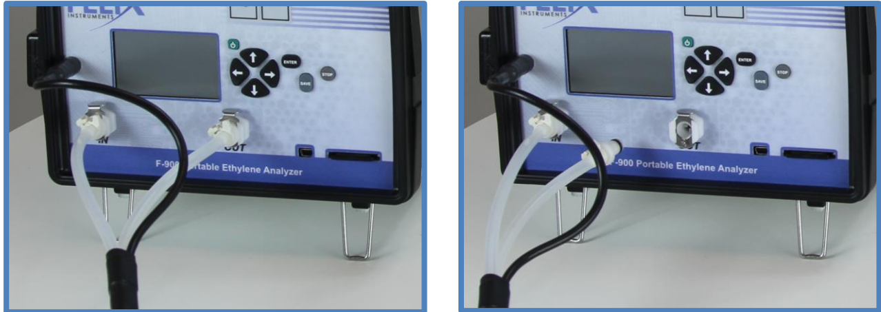
Figure 12: Using conditioned air to replenish the fruit chamber by connecting the IN and the OUT (left); using ambient air to replenish the fruit chamber by disconnecting the OUT (right).
