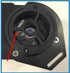
After the small fruit adaptor is installed, center the small fruit specimen on the central ring. This small ring will hold the fruit specimen in the correct position for measurements to be taken. Now, place the reflector cone over the specimen. You will notice that there are **magnets** installed within the reflector cone to obtain a good fit.
