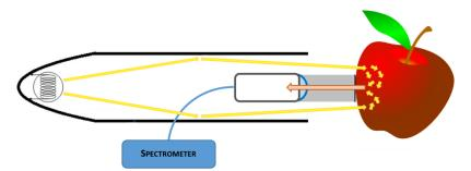
**Figure 1:** Interactance optical design; light rays illuminate an anulus on the sample. The light then interacts with the sample by internally scattering through the tissue. Light that undergoes remission normal to the collimating lens is collected and focused onto the fiber.
