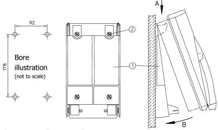
Figure 4: Mounting on a Wall
