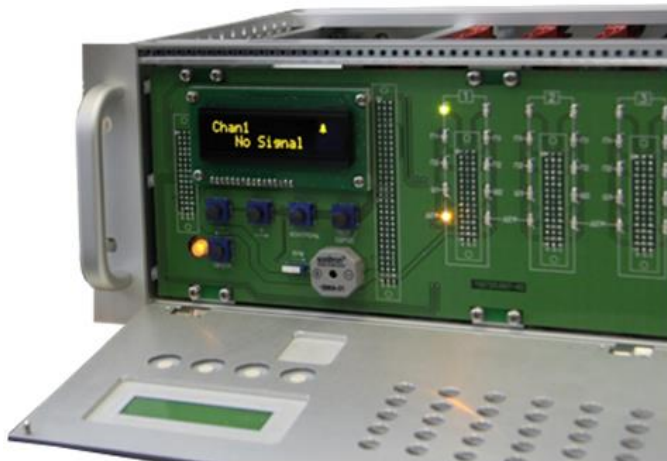
Fig.4.1. “No Signal” indication. Accompanied by audible alarm
