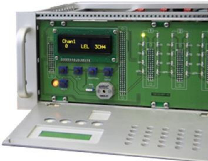
Fig.4. UPES-50A and gas detector standby mode
