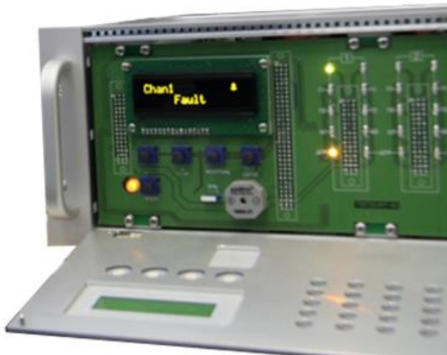
Fig. 3.3 When a magnet key is brought next to IPES, the device becomes faulty. UPES display indication is accompanied by audible alarm.
