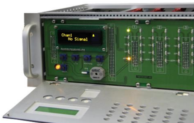
Fig. 3.4. UPES indication in case of loss of communication with IPES. Accompanied by audible alarm.
