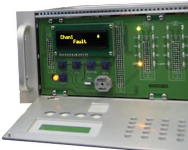
Fig. 3.2 IPES fault (dust condition), UPES indication fault display. Accompanied by audible alarm.
