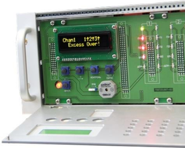
Fig. 4.5 “Excess Over” indication. Accompanied by audible alarm
