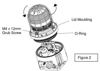
On completion of the installation the flameproof threaded joint should be inspected to ensure that they are clean and that they have not been damaged during installation. Flameproof threaded joints are not intended to be repaired. Also check that the 'O' ring seal is in place. When fitting the flameproof cover ensure the thread is engaged correctly. Fully tighten the cover all the way, ensure no gap is visible between the cover and base of the beacon enclosure. Tighten the M4 grub screw.
