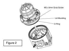
On completion of the installation the flameproof threaded joints should be inspected to ensure that they are clean and that they have not been damaged during installation. Flameproof threaded joints are not intended to be repaired. Also check that the 'O' ring seal is in place. When fitting the flameproof cover ensure the thread is engaged correctly. Fully tighten the cover all the way, ensure no gap is visible between the cover and base of the beacon enclosure. Tighten the M3 grub screw.
