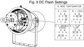
(Flip-Flop Mode not available on D1xC1X05 / D1xC2X05)
