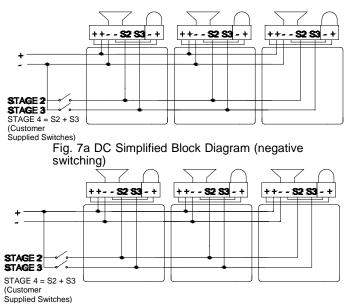
Fig. 7b DC Simplified Block Diagram (positive switching
