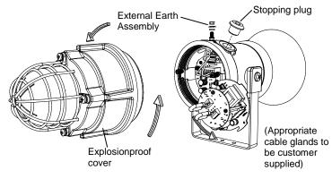
Fig. 2 Accessing the Explosionproof Enclosure.
