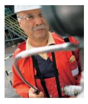
Dräger X-am 7000: Leak search made easy through the generation of a tracking sound.
