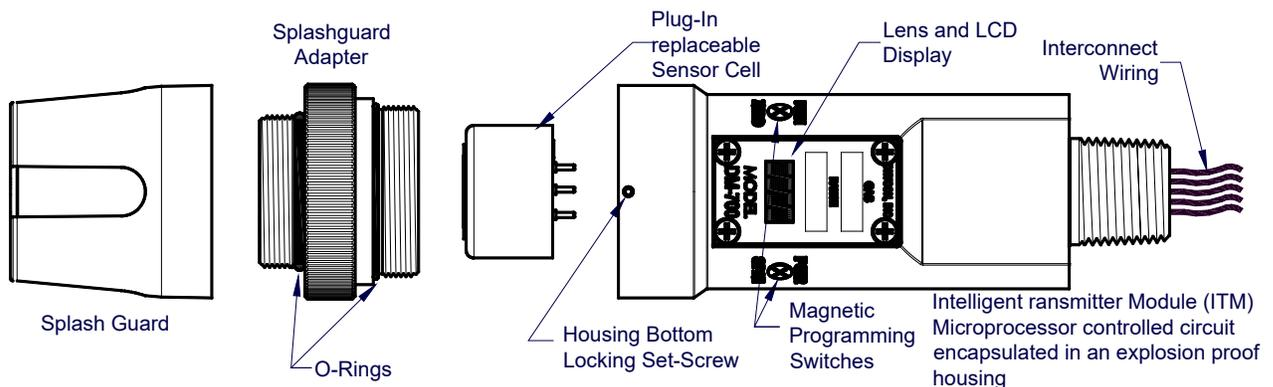
Figure 17 Sensor Assembly
