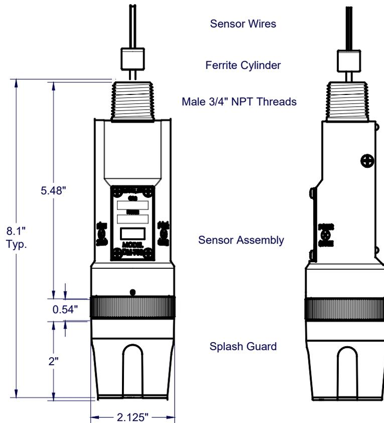
Figure 8 Outline and Mounting Dimensions (Sensor Assembly only)
