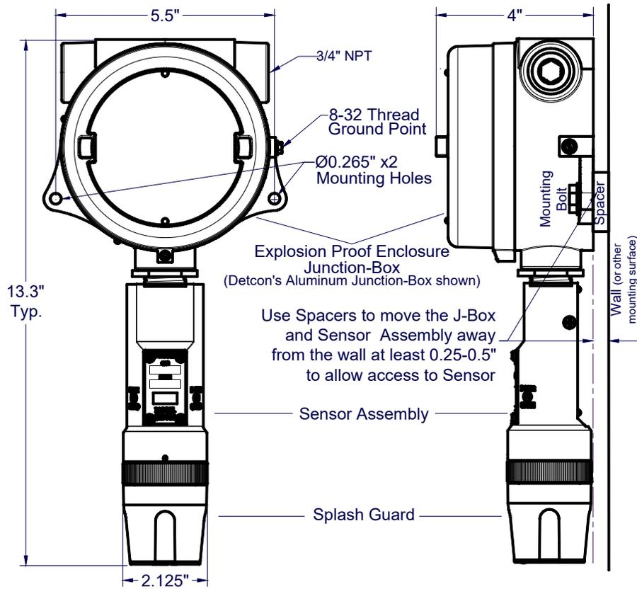
Figure 10 Outline and Mounting Dimensions (Aluminum Junction Box)
