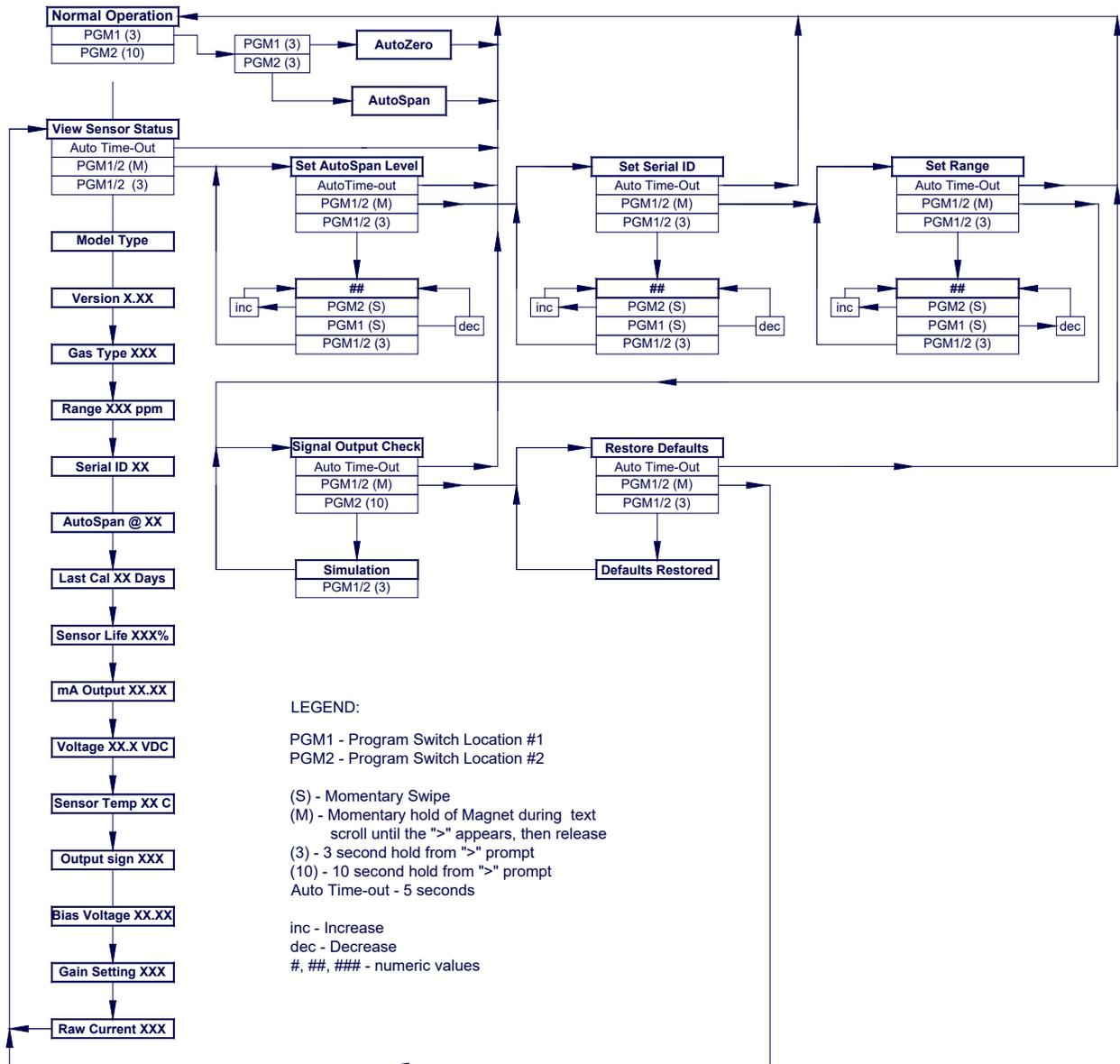
Figure 16 DM-700 Software Flowchart
