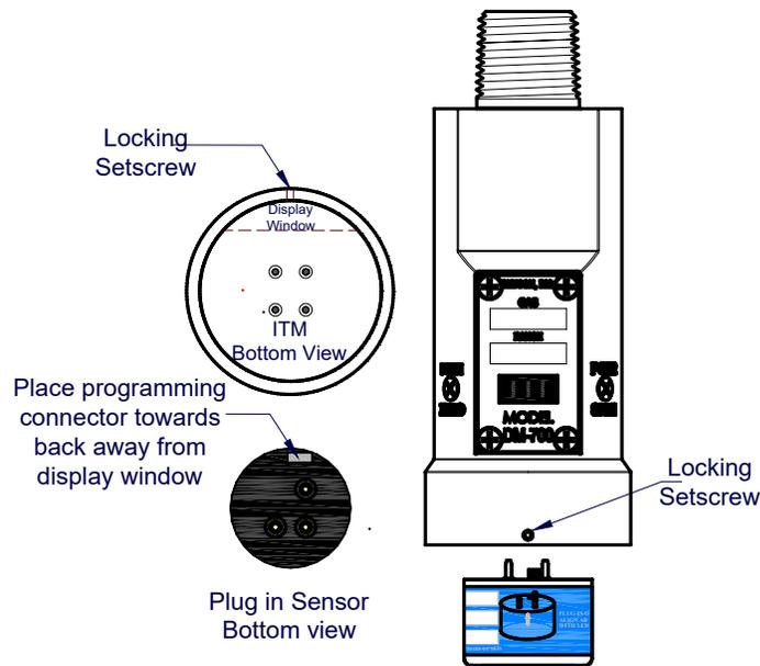
**Figure 18** Sensor Cell and ITM Mating
