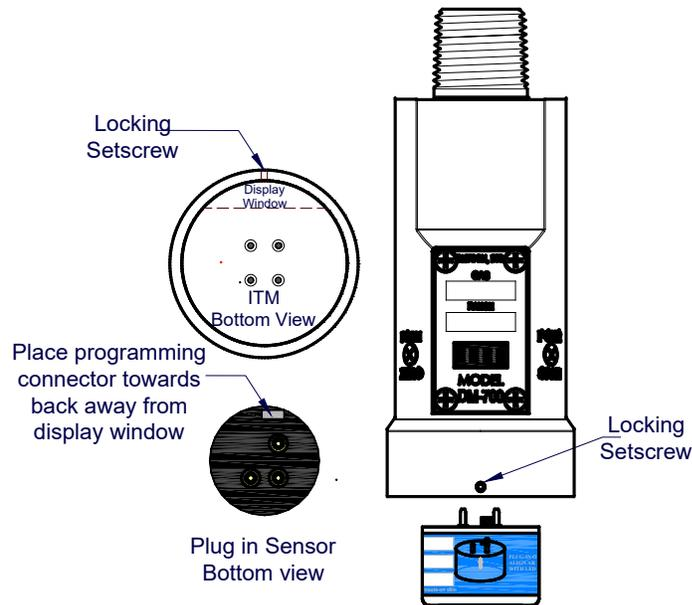
**Figure 19** Sensor Cell and ITM Mating
