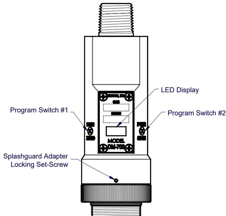
**Figure 15** Magnetic Programming Switches
