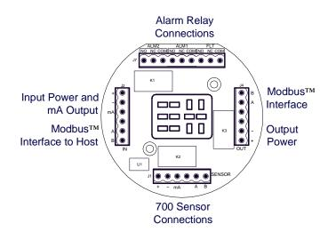
Figure 5 Interface connections on terminal board
