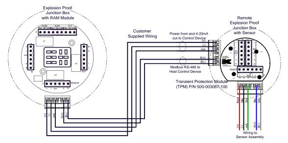
Figure 8 Remote Sensor Wiring
