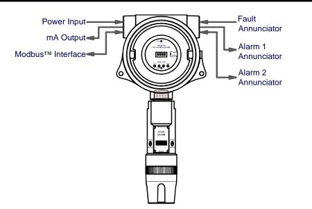
Figure 6 Installation with 700 Gas Sensor
