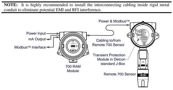
Figure 7 Remote 700 Gas Sensor with RAM
