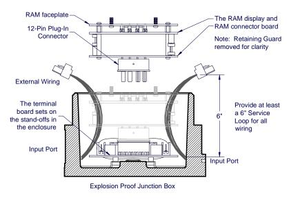
Figure 4 Exploded View of Assembly
