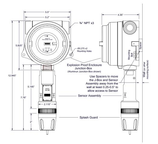
Figure 3 Mounting RAM with 700 Sensor
