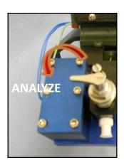
Figure 8.1-3: Close the valve to the ANALYZE position
