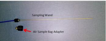
The air sample kit includes a sample wand and an air sample bag adapter. The air sample bag adapter enables direct connection to an air sample bag.
