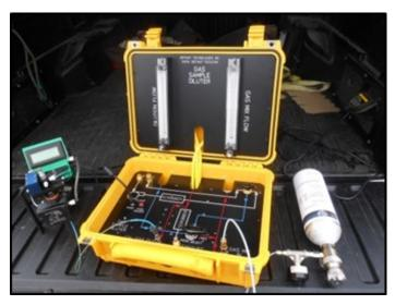
Gas Diluter attached to Calibration gas and FROG
