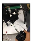
Connect the air sampler's valve connector to the FROG valve connection. This connection supplies power to the air sampler.
