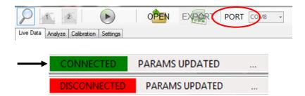
The connection status indicator in the lower left corner should now read CONNECTED indicating that the FROG and Ellvin are connected. The user may now manage settings and run analyses from Ellvin.
