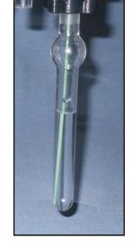
Figure 8.1-4: Look for Bubbles in the sparge bottle.
