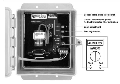
Figure 3: Sensor board components and zero/span adjustments
