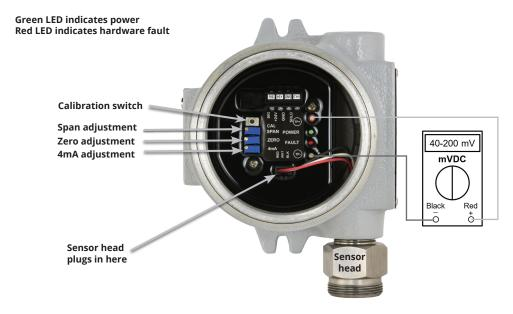
Figure 2: Sensor output and zero/span adjustment
