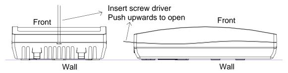
Figure 1. Closed housing seen from the top and the side. The housing is opened by inserting a screw driver and pushing to the front side of the housing. The locking hooks will then be released.
