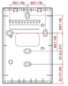
Figure 3. The dimensions of the sensor in mm and (inches)
