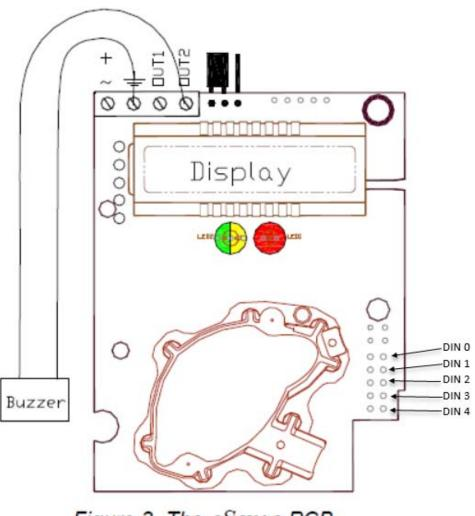
Figure 3. The eSense PCB
