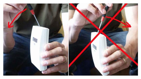
Figure 2. Closed housing seen from the side. The housing is opened by inserting a screwdriver and pushing left (to the front side).
