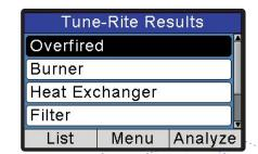
display a prioritized list of most likely potential issues to investigate. A drill-down into a "checklist" helps to keep track and record what has been inspected, adjusted, repaired or found to be an issue.
